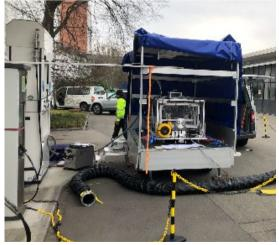
The H2 MOBILITY metering device allows for calibrating stations during ongoing operation  $\dots$
